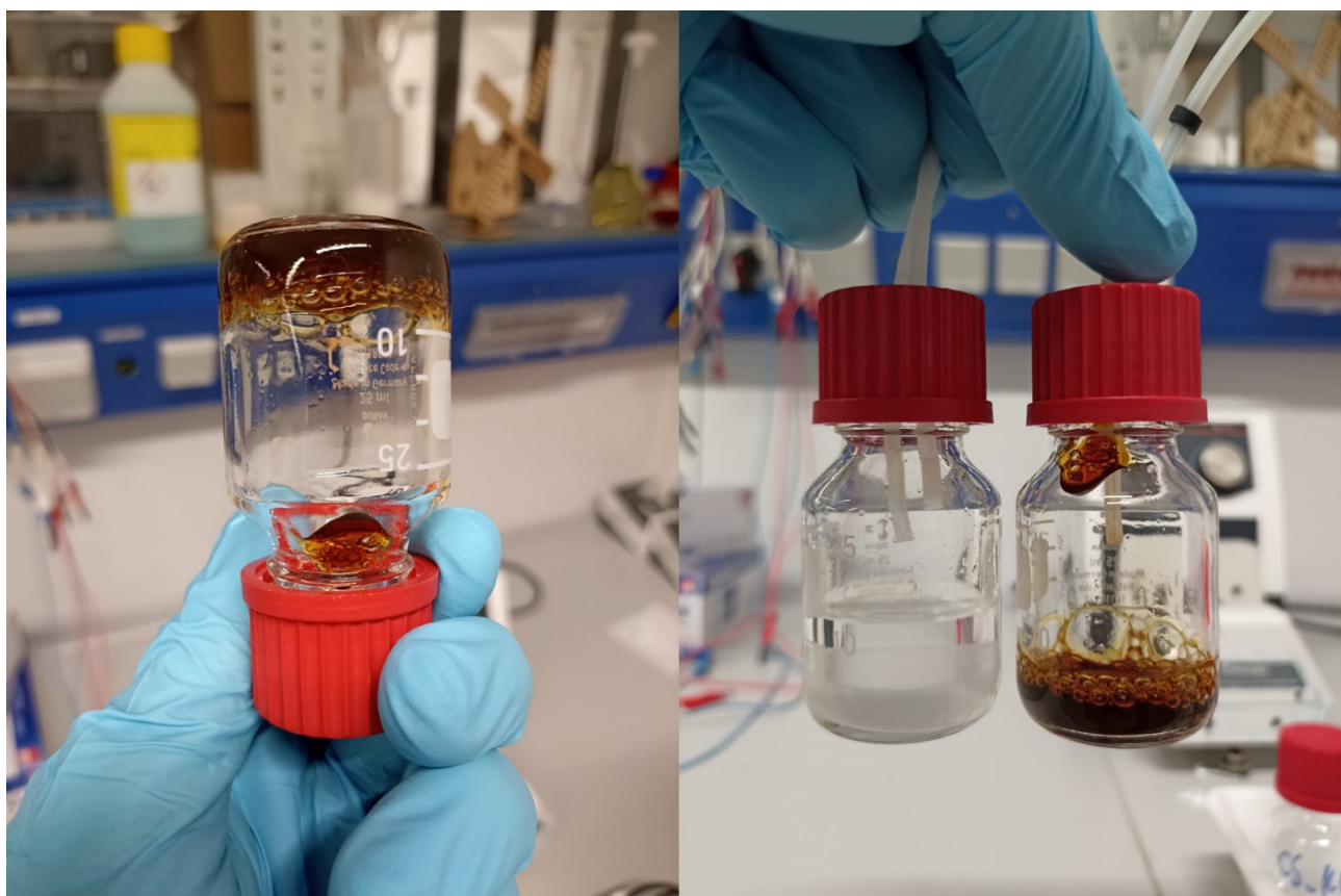
Figure S9 Photographs of RFB electrolytes after the battery cycling under ambient conditions, outside the glovebox. Conditions: Continuous battery cycling of 10 ml 27 mM PFC, 0.1 M \text{ZnCl}_2 , 0.8 M \text{NH}_4\text{Cl} catholyte vs. 10 mL 0.1 M \text{ZnCl}_2 , 0.8 M \text{NH}_4\text{Cl} anolyte galvanostatically at 16 \text{ mA cm}^{-2} current in a 0.5 to 1.5 V cutoff voltage range with subsequent potentiostatic holding at cutoff voltages till absolute current value decreases to \leq 0.5 \text{ mA cm}^{-2} . Strong osmosis caused water transfer into the anolyte.
