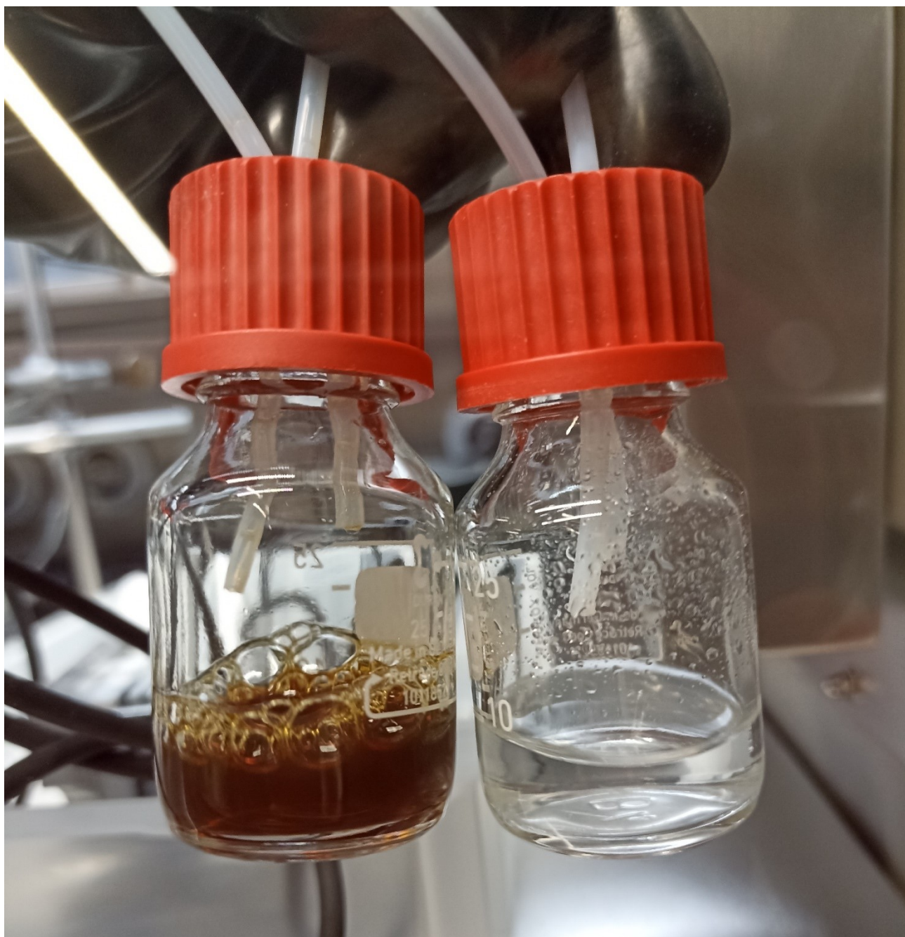
Figure S10 Photograph of the RFB electrolytes after battery cycling in the glovebox. Conditions: Continuous battery cycling of 10 mL 27 mM PFC, 0.1 M \text{ZnCl}_2 , 0.8 M \text{NH}_4\text{Cl} catholyte vs. 10 mL 0.1 M \text{ZnCl}_2 , 0.8 M \text{NH}_4\text{Cl} anolyte galvanostatically at 16 \text{ mA cm}^{-2} current in a 0.5 to 1.5 V cutoff voltage range with subsequent potentiostatic holding at cutoff voltages till absolute current value decreases to \leq 0.5 \text{ mA cm}^{-2} .
