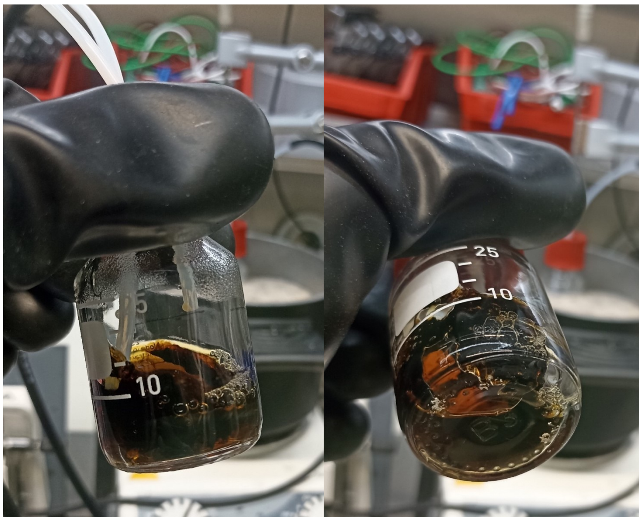
Figure S44 Gel phase formed at the catholyte tank walls during the full RFB thermal assessment test at 60 °C (setup 3).
