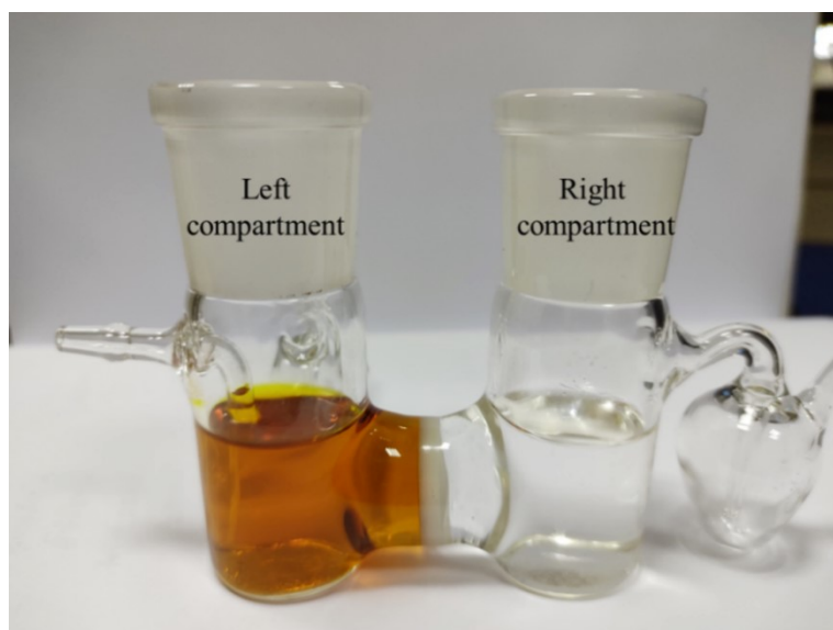
Figure S17 H-cell setup for the controlled potential electrolysis experiment [The working chamber at the left contains 0.5 mM catalyst, 100 mM n\text{-Bu}_4\text{NPF}_6 , 100 mM phenol, THF, and the counter chamber at the right contains THF, 100 mM n\text{-Bu}_4\text{NPF}_6 .
