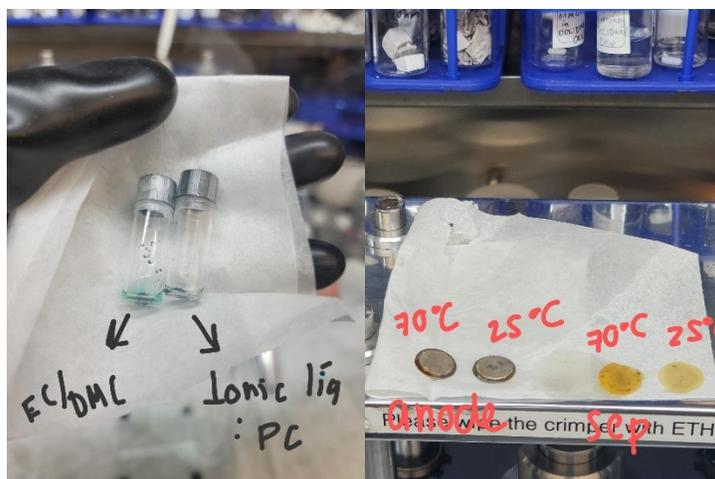
**Figure S3.** Left panel shows the dissolution of  $\text{VO}_2(\text{M})$  into the EC: DMC organic electrolyte system (blue coloration) compared to no coloration in the ionic liquid electrolyte. Right panel shows the re-oxidation of  $\text{VO}_2$  to  $\text{V}_2\text{O}_5$  (characterized by its yellow coloration) and dissolution into the electrolyte at room and elevated temperatures.
