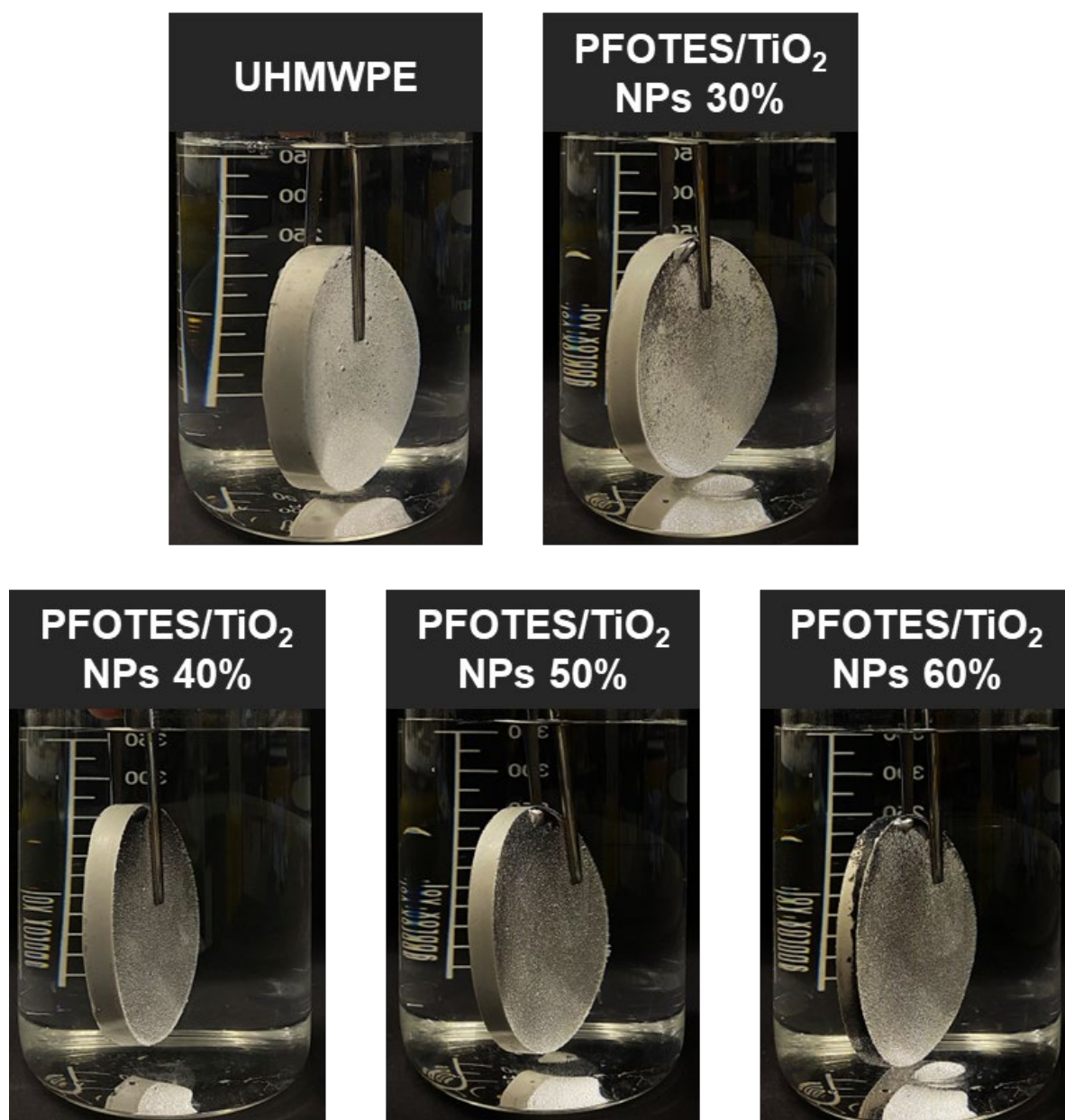
Fig. S10 Plastron effect of UHMWPE and composites containing 30, 40, 50 and 60% PFOTES/TiO 2 NPs which have a water contact angle of >150^\circ . The samples with a S_a of >16\ \mu\text{m} were used for the plastron effect test.
