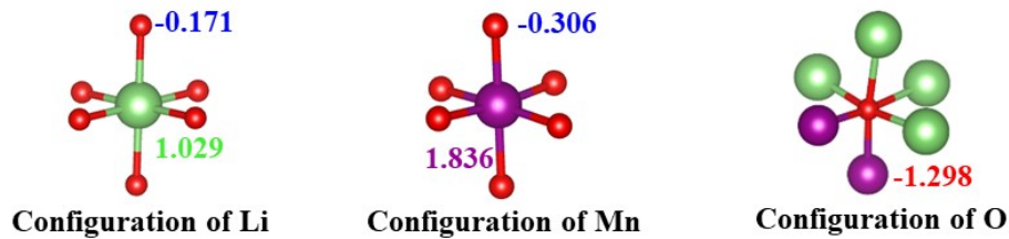
Fig. S17. The coordination environment of various atoms in Li_2MnO_3 bulk structure. The green, purple, and red fonts represent the average Hirshfeld-I charges of Li, Mn, and O in the bulk structure, respectively, and the blue font represents the average Hirshfeld-I charges provided by Li ion or Mn ion to surrounding O ions (Green: Li; Purple: Mn; Red: O).
