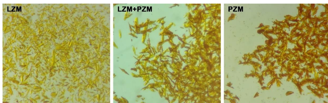
Figure S1. Optical micrograph images showing phase transition from LZM to PZM. The samples in the figures (from left to right) correspond to the addition of LZM (5 mg) and bpy (50 mg) in DMF/H 2 O (4.5 mL) at 100 °C for 0, 3 and 5 days, respectively.
