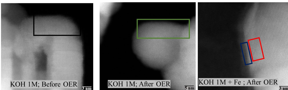
Figure S6. STEM images of \text{LaNiO}_3 under different conditions. The EELS spectra are collected from the respective marked regions; before OER (black colour), after OER in 1M KOH (green colour), nanoparticles after OER in 1M KOH with Fe impurities, the amorphous layer formed after OER in 1M KOH with Fe impurities.
