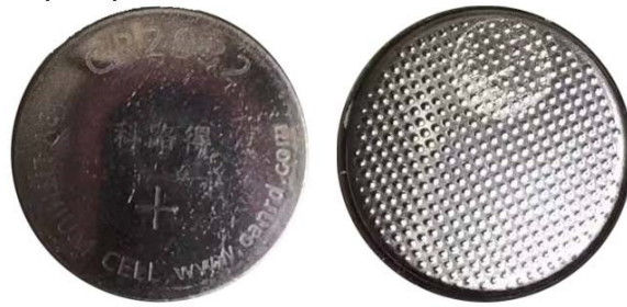
Fig. S11. The assembled prototype of the supercapacitor.
