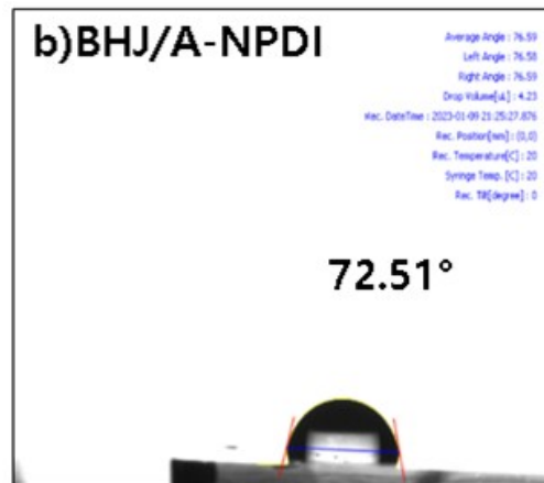
Fig. S12. DI water contact angle analysis of BHJ with (a) conventional NPDI and (b) coherent arrangement NPDI films.
