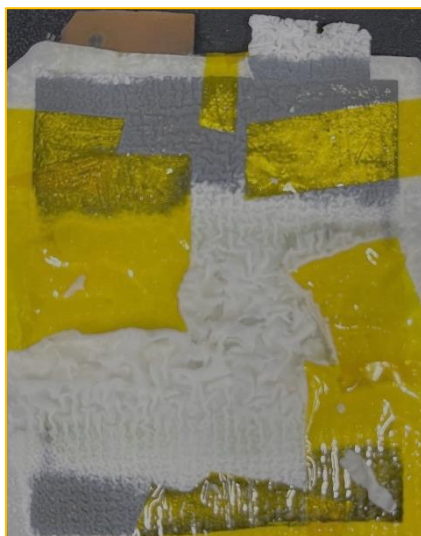
Figure S35. Optical photograph of Lithium foil corresponding to the dissected flexible quasi-solid-state Li-CO 2 pouch battery with the Fe 2 O 3 /Cu 2 O/Cu nanowires cathode after cycle test at a current density of 0.05 mA·cm -2 .
