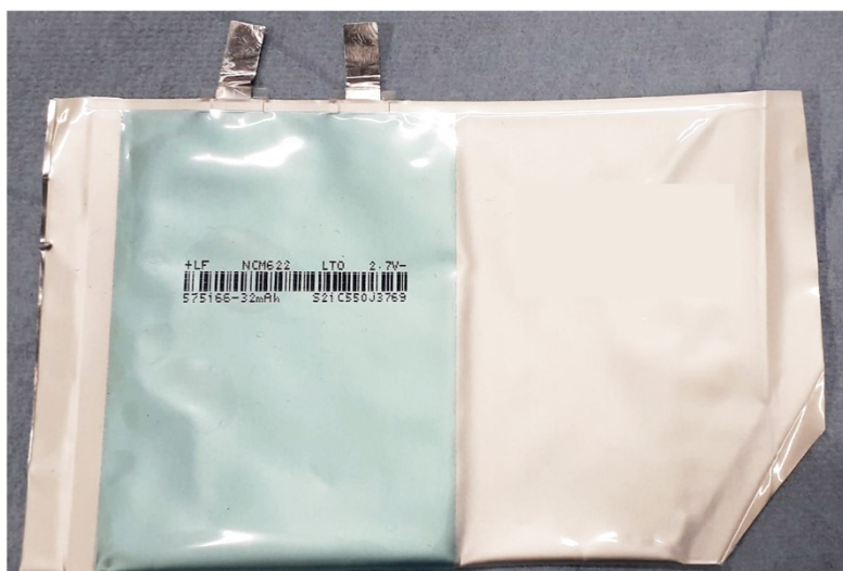
SI Figure 6: Photograph of the commercial LTO-NMC622 commercial cell supplied from LiFun, after extensive cycling and before manual dismantling.
