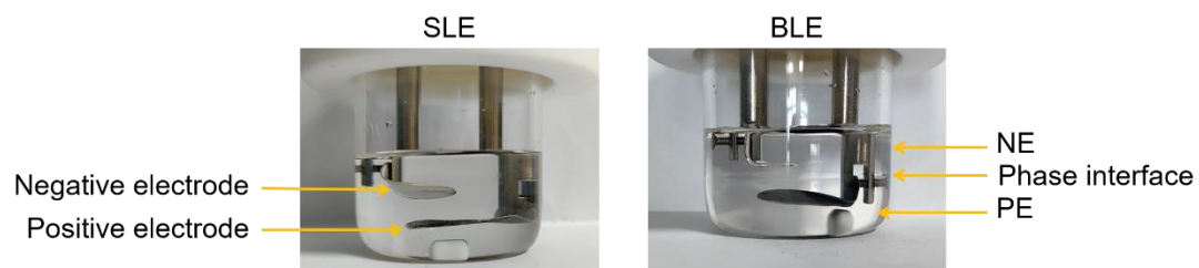
Fig. S14 The structure of beaker cells with the SLE (1 M LiTFSI in G4, left) and BLE (1 M LiTFSI in G4/EGDE (v/v = 5/5), right). Lithium foil and CNTs were used as the negative and positive electrode, respectively.
