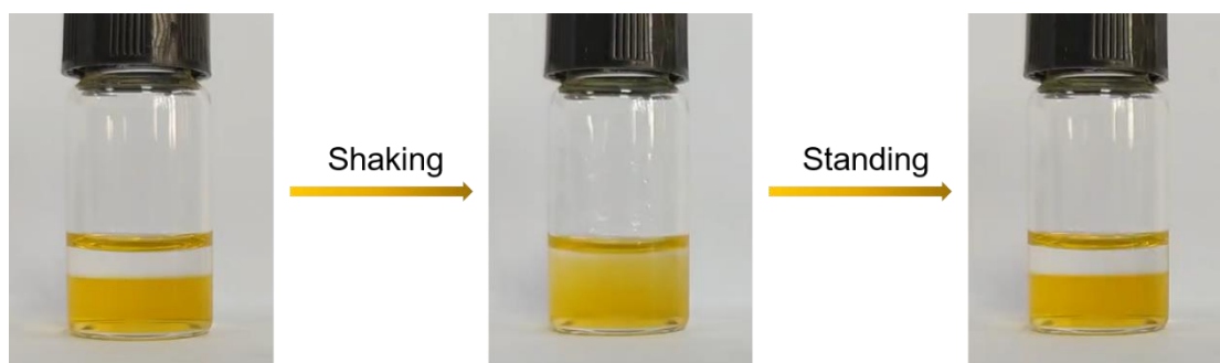
Fig. S11 Optical images of ether/ether based BLE with 20 mM \text{Br}_3^- as a color indicator after violent shaking.
