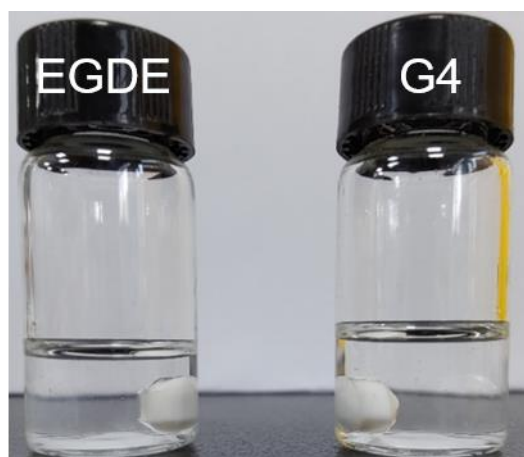
Fig. S2 Optical images of G4 and EGDE based electrolyte with maximum LiTFSI solubility. The concentration of LiTFSI in EGDE is up to 4.0 M (Left), and the concentration of LiTFSI in G4 can reach 6.0 M (Right).
