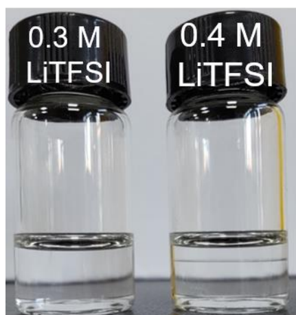
Fig. S5 Optical images of G4 and EGDE mixed solution (G4/EGDE (v/v = 5/5)) with 0.3 M LiTFSI (Left) and 0.4 M LiTFSI (Right).
