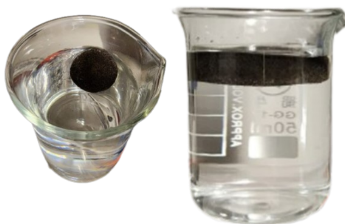
Self-floating capability of OPU
