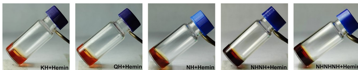
Fig. S16 Optical images of the peptide-hemin (molar ratio 10:1) hydrogels from KH_{\text{hemin}} (0.1 wt%, pH 7.4), QH_{\text{hemin}} (3.0 wt%, pH 7.4), NH_{\text{hemin}} (0.5 wt%, pH 7.4), NHHH_{\text{hemin}} (0.8 wt%, pH 7.4), and NHHHHH_{\text{hemin}} (0.8 wt%, pH 7.4), respectively.
