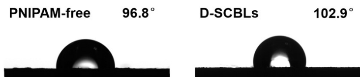
Fig. S10 Water CAs of the PNIPAM-free surface and D-SCBLs.
