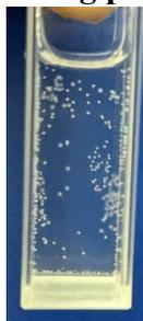
Fig S14: Tiny H<sub>2</sub>S bubbles formation during photolysis of BCS solution
