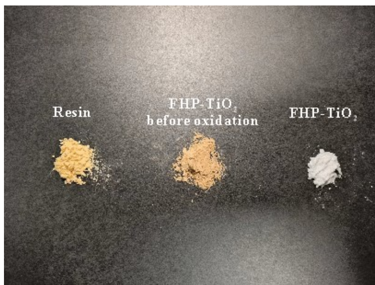
Figure S9. Image of FHP-TiO 2 before and after oxidation.
