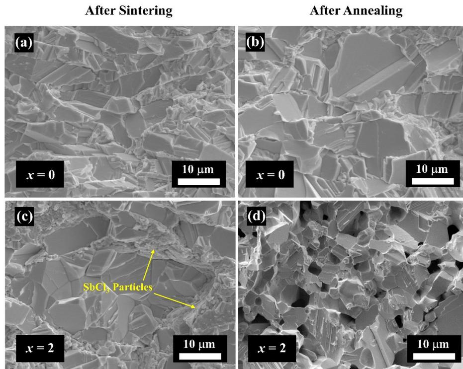
Fig. S4 FESEM images of fractured surface of (a, c) the sintered  $x = 0, 2$  samples and (b, d) the annealed  $x = 0, 2$  samples, respectively.
