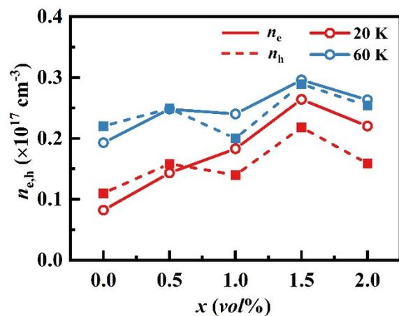
Fig.S7 Electron and hole concentration as a function of  $x$  at 20 and 60 K for  $\text{Bi}_{0.85}\text{Sb}_{0.15}/x$  vol% $\text{SbCl}_3$  porous samples, respectively.
