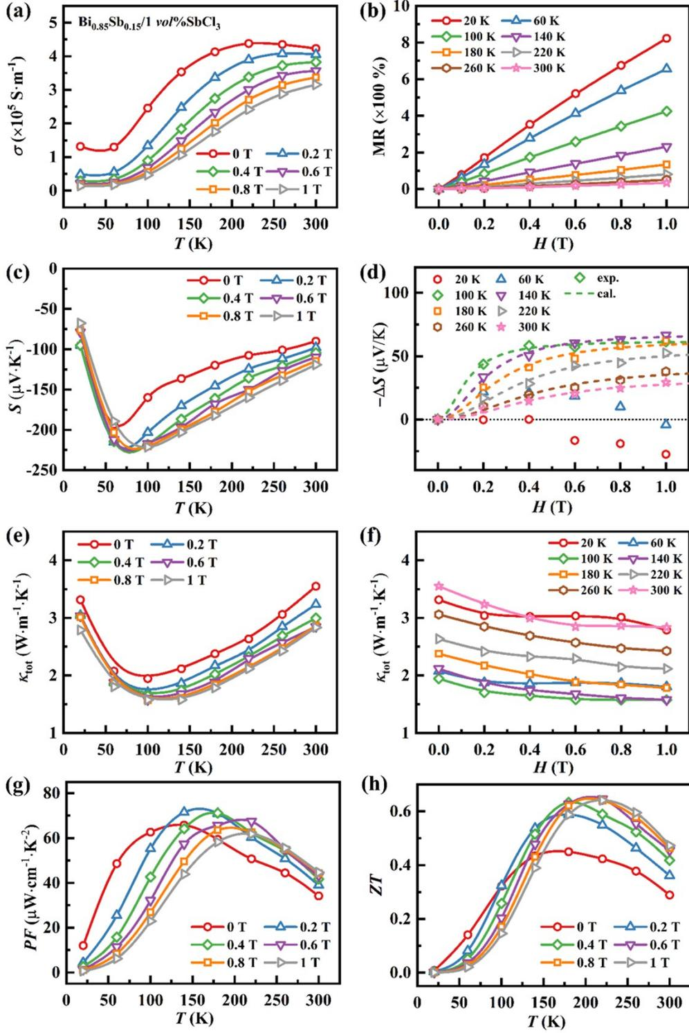
Fig.S10 Thermoelectric properties of  $\text{Bi}_{0.85}\text{Sb}_{0.15}/1 \text{ vol}\% \text{SbCl}_3$  sample in the magnetic field of 0-1 T. Temperature dependence of (a) conductivity, (c) Seebeck coefficient, (e) thermal conductivity, (g) power factor, and (h)  $ZT$  values, respectively. Magnetic field dependence of (b) conductivity, (d) Seebeck coefficient, (f) thermal conductivity, respectively.
