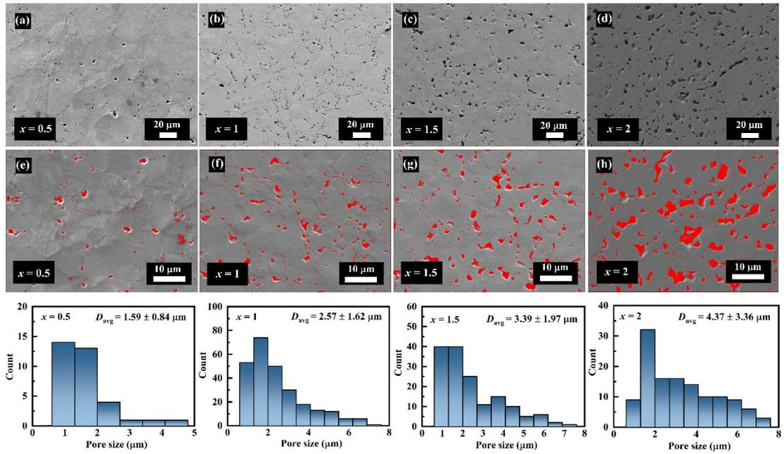
Fig. S3 (a-d) FESEM images of polished surface of the  $x = 0.5, 1, 1.5, 2$  sample, respectively. (e-h) The built-in Pore size of the  $x = 0.5, 1, 1.5, 2$  sample, respectively (The pores are filled with the red color to guide the eye).
