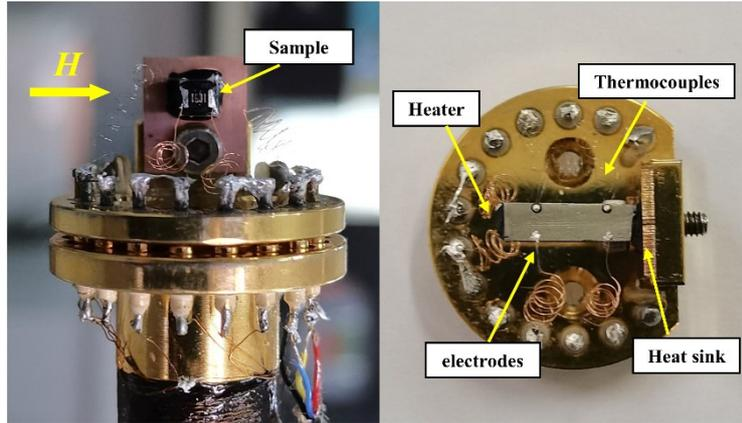
Fig.S1 Typical image of the sample mounting for TE parameters measurements.
