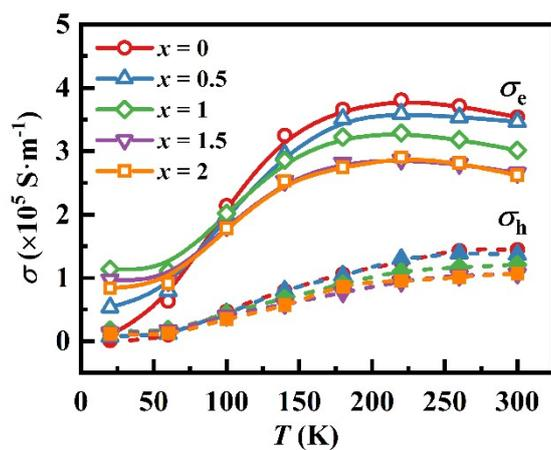
Fig.S8 Temperature dependence of partial electron (hole) conductivity of  $\text{Bi}_{0.85}\text{Sb}_{0.15}/x$  vol% $\text{SbCl}_3$  porous samples.
