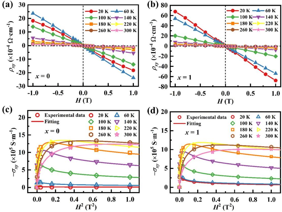
Fig.S6 Magnetic field dependence of (a,b) Hall resistivity and (c,d) magnetoconductivity at various temperature for  $x = 0$  and  $x = 1$  sample, respectively.
