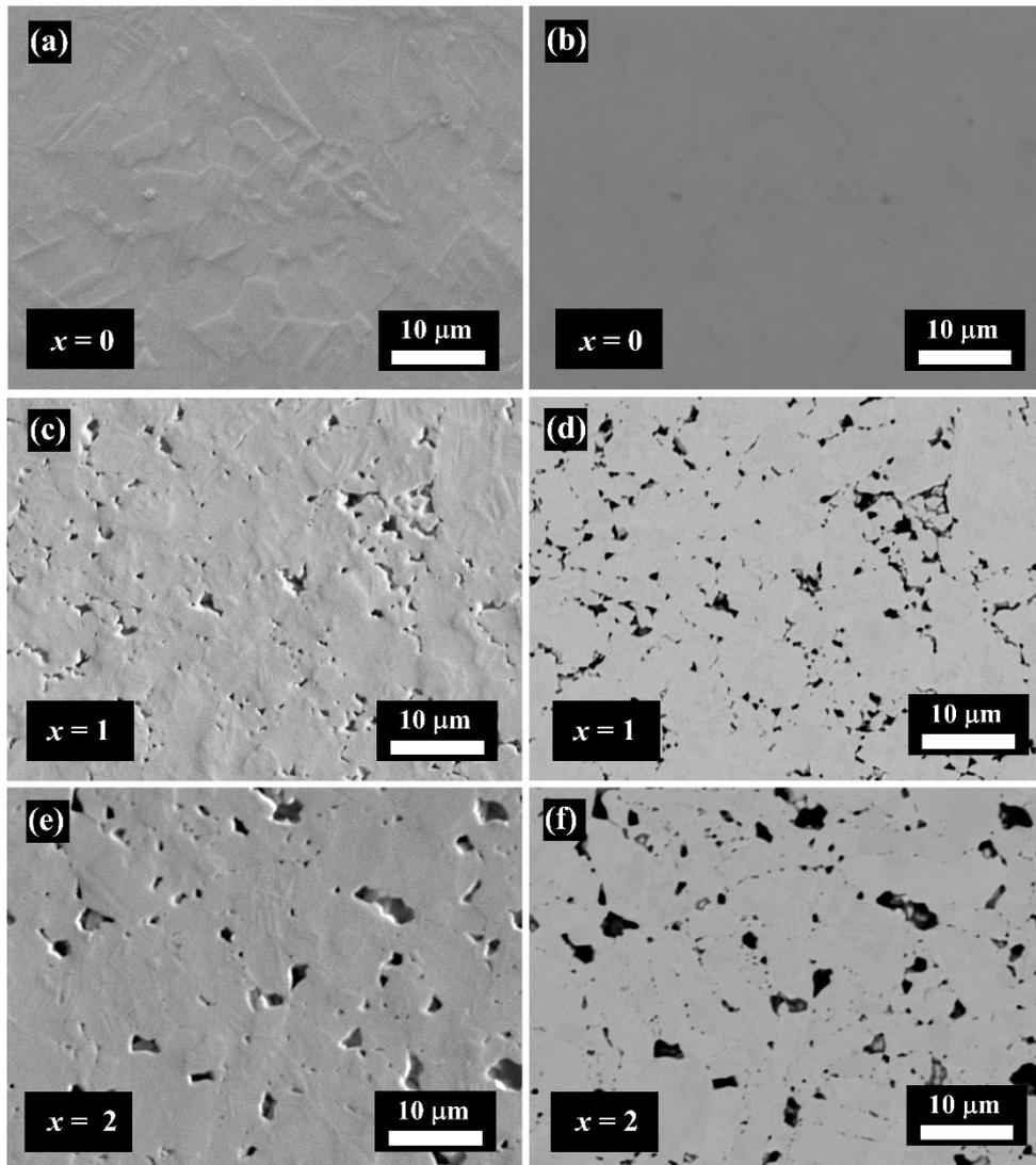
Fig. S2 (a, c, e) FESEM images and (b, d, f) corresponding BSE images of polished surface of the  $x = 0.5, 1, 2$  sample, respectively.
