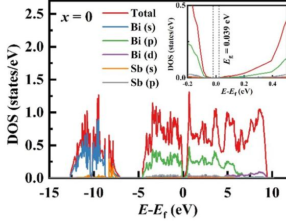
Fig. S5 The calculated projected electronic DOS of  $x = 0$  sample.
