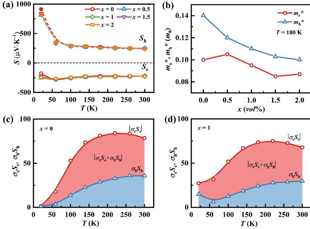
Fig.S9 (a) Temperature dependence of partial electron (hole) Seebeck coefficient of Bi<sub>0.85</sub>Sb<sub>0.15</sub>/x vol% SbCl<sub>3</sub> porous samples. (b) The estimated effective mass of electron and hole at 180 K. (c,d) Temperature dependence of  $(\sigma_e S_e, \sigma_h S_h)$  term for the  $x = 0$  and  $x = 1$  samples, respectively.
