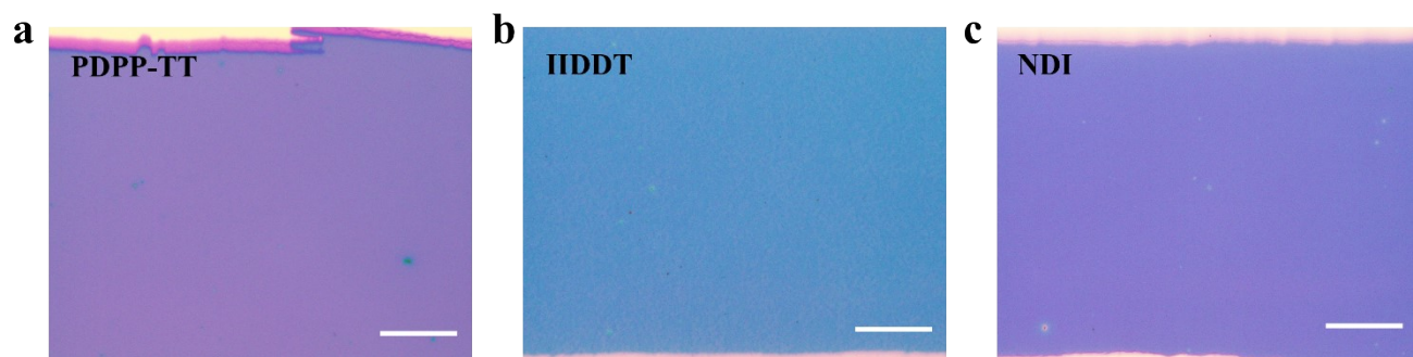
Fig. S1. Optical microscope (OM) images of pristine (a) PDPP-TT, (b) IIDDT and (c) NDI semiconductor films. The scale bar is 10 \mu\text{m} .
