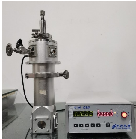
Figure S1. Cryogenic control equipment. Cooperate with the fluorescence spectrometer to realize temperature-dependent spectra testing.
