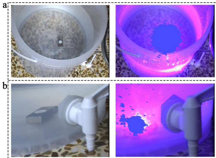
Figure S2. Demonstration of tagging via SrSiO 3 :0.02Pr 3+ in a bucket by using a 450 nm LD as excitation source. (a) Top view, and (b) Side view. Left panel: under natural light, and right panel: under excitation of a 450 nm LD.
