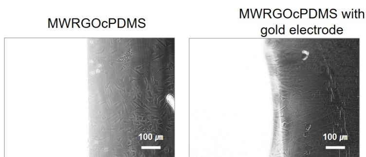
Figure S14. Microscopic images harvested with a stronger illumination. L929 fibroblasts were exposed with the MWRGOcPDMS graphene sensors without gold electrode (left) and with gold electrode (right) for 24 h. The scale bars are 100 \mu\text{m} .
