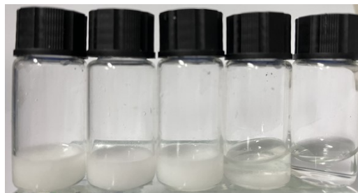
Figure S2. The gelation of different DMSO content solutions. The DMSO content was 10 %, 20 %, 30 %, 40 % and 50 % from left to right, respectively.
