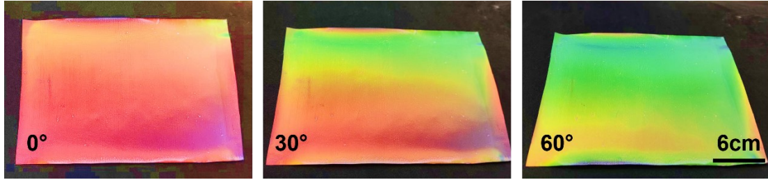
Figure S2 Angle-dependent structural colors of PMMA photonic crystals on fabric substrate.
