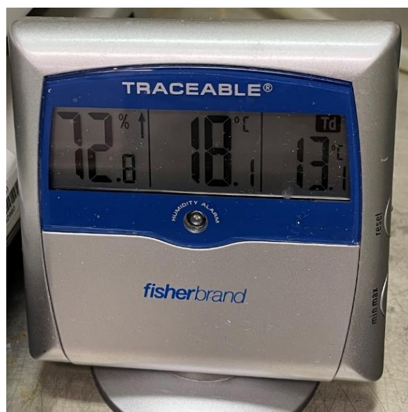
Figure S1 Humidity meter showing relative humidity 72.8% during the fabrication of the PSCs.
