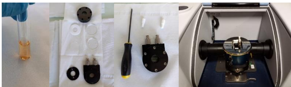
Figure S17. The YELLOW CNDs in the d_6 -DMSO suspension (a), the construction of the CaF 2 liquid cell (b-c), and the view of the sample chamber in the IR spectrometer working in the transmission mode (d).
