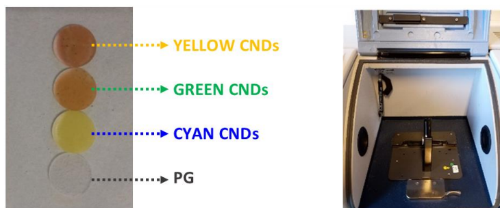
Figure S16. The analytes in KBr pellets (a) and the sample chamber in the IR spectrometer operating in the transmission mode (b).
