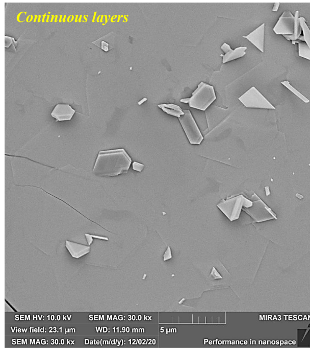
Figure S1. \text{Bi}_2\text{Se}_{(3-x)}\text{S}_x morphologies by SEM images on various substrates: (a) Si/SiO 2 , (b) sapphire, and monolayer graphene on Si/SiO 2 grown for (c) 60 minutes, (d) 120 minutes, and (e) 180 minutes.
