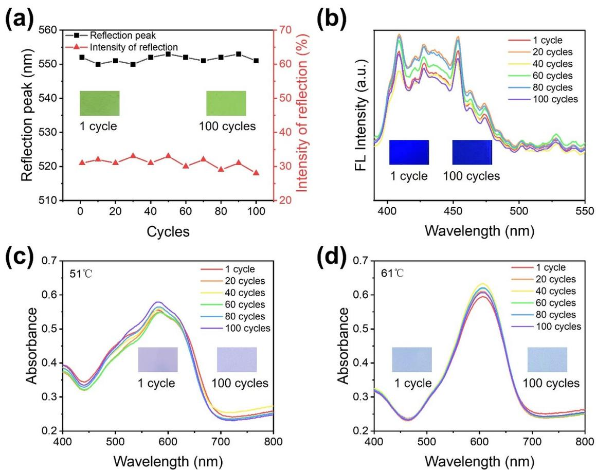
**Fig. S9** Reusability and stability of the PCC films after undergoing 100 cycles. (a) Reflection peak and intensity, (b) fluorescent luminescence, (c) absorption spectra at 51 °C, and (d) at 61 °C.
