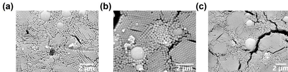
**Fig. S6** Top-view SEM images of the PCC film including P(St-MMA-AA) nanospheres, thermochromic microcapsules, and 2-AC.
