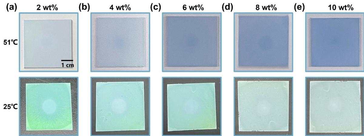
**Fig. S2** Photographs of the PCC films with different mass fractions of blue thermochromic microcapsules. It is shown that the color of PCC film displayed both saturated blue color at 51 °C and brilliant green color at 25 °C when the doping content was 6 wt.%. In this regard, the mass fraction of the colored microcapsules was kept at 6 wt.% if not stated otherwise in this work.
