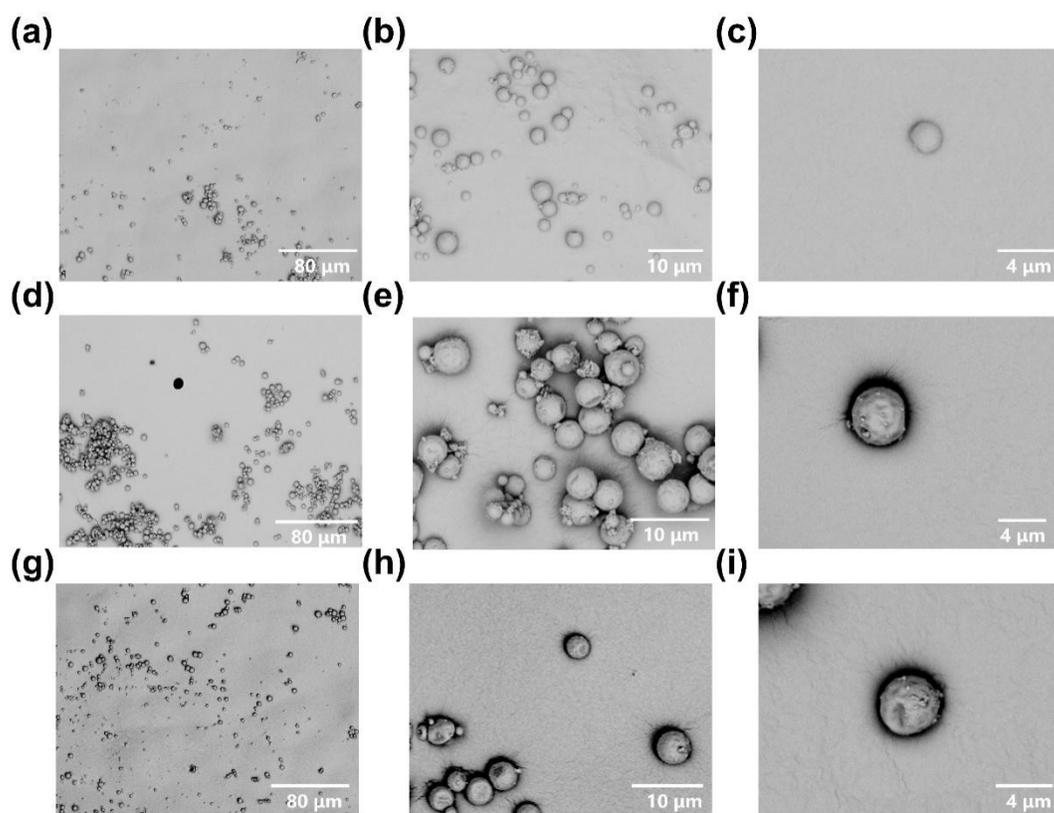
**Fig. S5** Top-view SEM images of the thermochromic microcapsules. (a-c) black, (d-f) purple, and (g-i) blue microcapsules.
