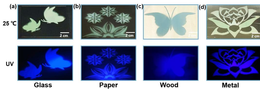
**Fig. S7** Photographs of patterned PCC films at 25 °C and UV illumination on various substrates.
