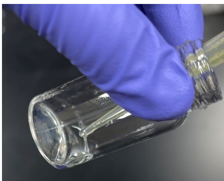
Figure S12. Magnified photograph of MAPbBr 3 -PU (1.7 wt%) solution. The PU precipitates form a large lump, separated from the solution.
