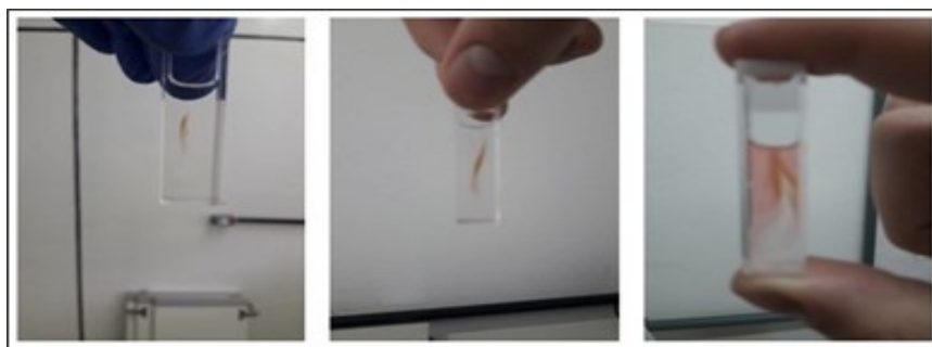
Figure S15. Pictures taken at 5, 10 and 15 min irradiation of the DaO in THF, ( [DaO] = 1.0 \times 10^{-3} M ).
