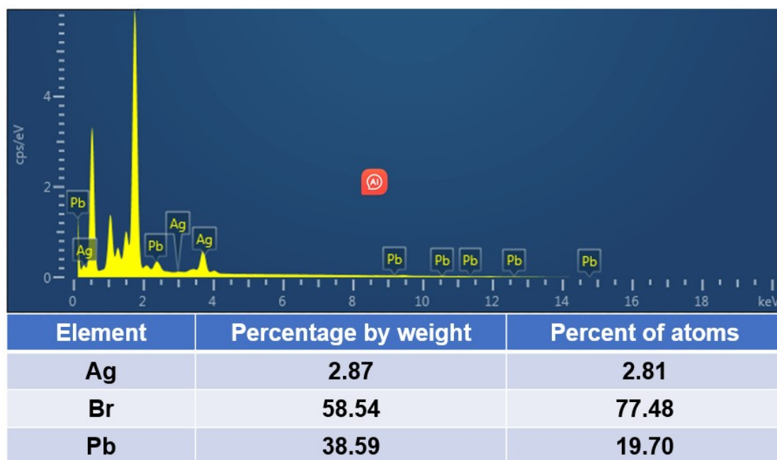
Figure S5. Element distribution of MAPbBr 3 crystal in Figure S4d .
