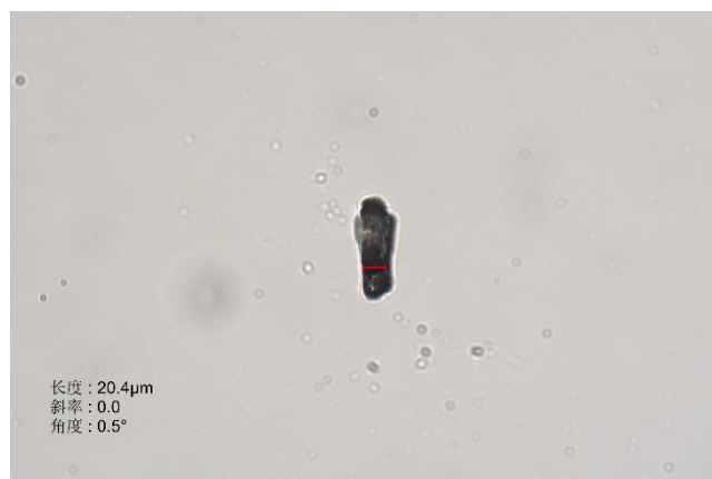
Figure S3. Crystal used for birefringence measurements with thickness of 20.4 \mu\text{m} .
