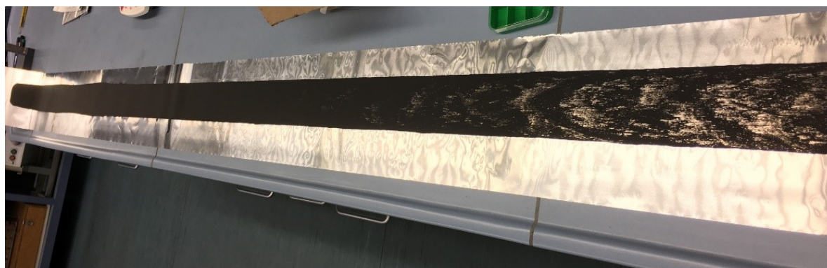
Figure S-2. Gelation hindering continuous processability while coating the additive-free 70 mass% SC cathode slurry.
