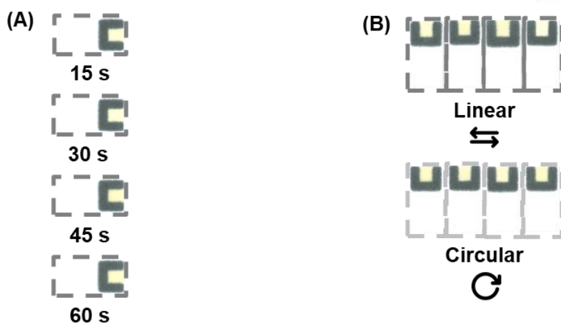
Fig. S2 Optical images showing the captured data for the optimization of time and type of mixture. (A) PADS and graph of the variation of the mixing time in the circular model by the corresponding color intensity and (B) PADS and graph comparing the circular and linear mixture in 45 s by the corresponding color intensity.
