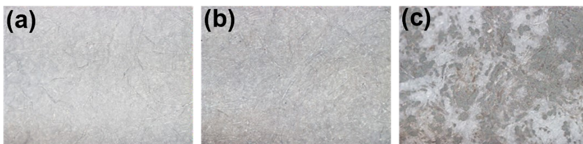
Figure S1 OM images reveal the surface of the filter paper after filtration with (a) colloidal PSNs, (b) colloidal AgNPs, and (c) PSNs/AgNPs with MgCl_2 as aggregating agents.
