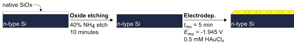
Figure S1. Schematic showing the fabrication of n-Si/metal LAE sensors prepared using electrodeposition.
