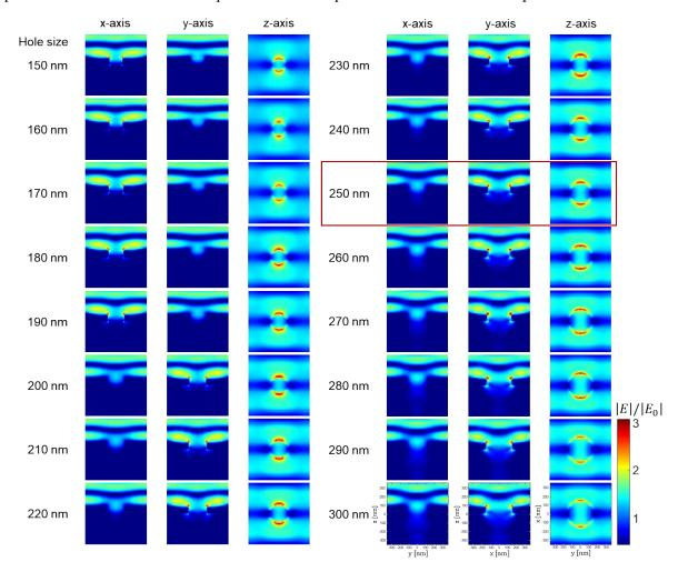
The results confirm increased localization as the nanohole diameter  $\phi$  decreases, which is especially clear in the *xy*-plane (*z*-axis). The peak electric field amplitude does not exhibit a significant or monotonic change.
