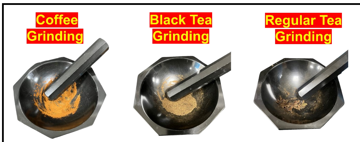
Figure S5. Camera images of grinding of coffee, black tea, and regular tea for XRD measurement.
