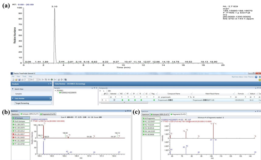
Fig. S1. Example of fast screening and identification of propamocarb [M+H]^+ ( m/z 189.15975; t_R = 3.10 min) in solvent at 2 \text{ mg L}^{-1} using Thermo Xcalibur software. The identification of propamocarb in sample was defined on the basis of t_R variation, accurate mass measurement, fragment ions, and isotope peak. (a) Extracted ion chromatogram of propamocarb; (b) Experimental isotopic pattern (in blue) against a theoretical pattern based on the elemental composition and adduct (in red); (c) Product ion spectrum (in blue) matched against the pesticides of in-house database using solvent (in red).
