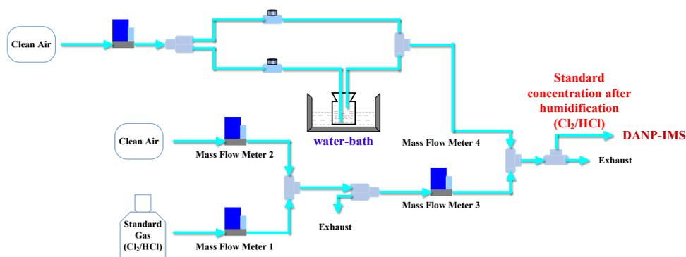
Fig S2. Schematic diagram of the online dilution and humidification system.
