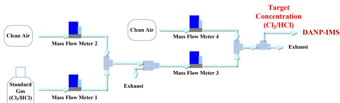
Fig S1. Schematic diagram of the online dilution system.
