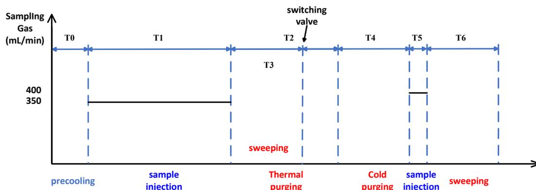
Fig S3. Working sequence of DANP-IMS coupled semiconductor cooling pre-processing method.
