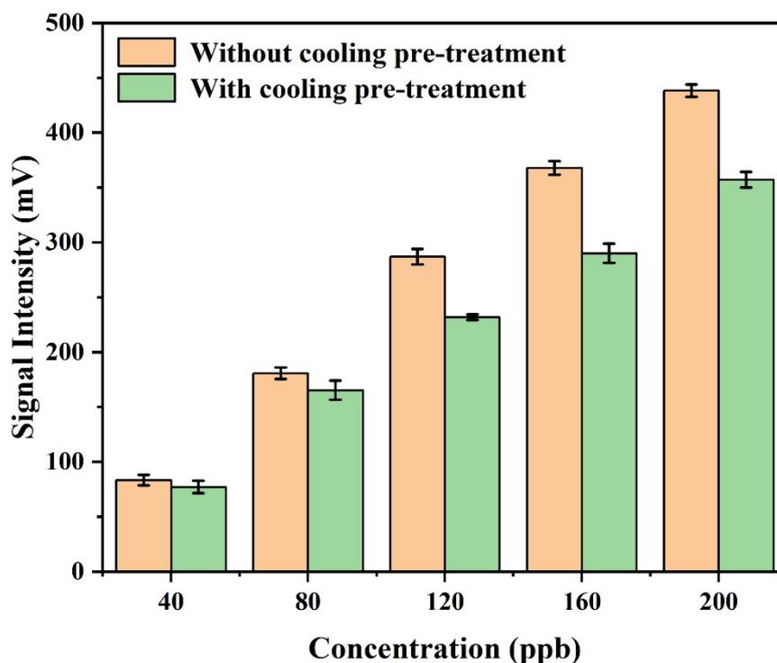
Fig S4. Comparison of signal intensity of Cl<sub>2</sub> passing through the cold trap and not passing
