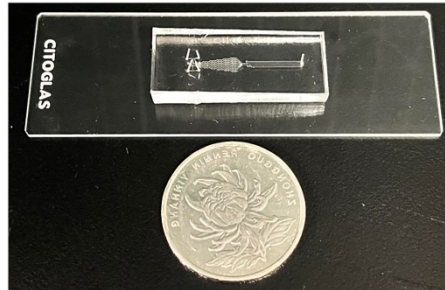
Fig. S2. Schematic representation of the microfluidic design and real picture of the proposed microfluidic chip.
