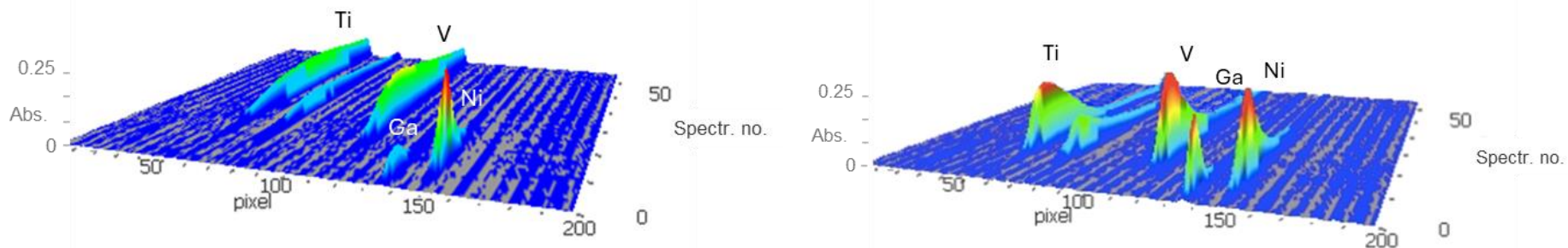
Fig. SM2. Time resolved absorbance spectra obtained by HR CS GFAAS measurement for 150.0 \mu\text{g L}^{-1} V, Ti, 300 \mu\text{g L}^{-1} Ni and 15 \mu\text{g L}^{-1} Ga (A) without Nb coating, spectral range between 294.1349 and 294.4999 nm; (B) with Nb coating, spectral range from 294.1349 and 294.4999 nm
