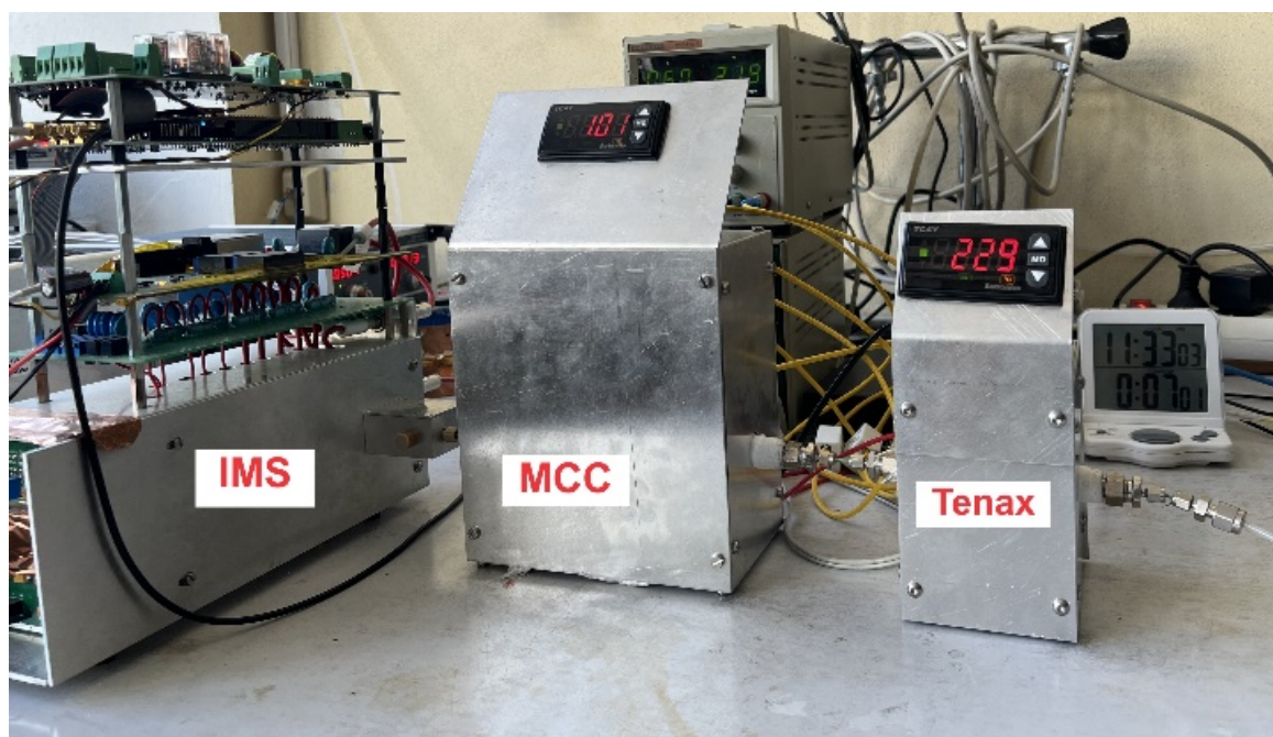
Figure S1. Experimental set up for detection of VOCs by Tenax-MCC-IMS. The VOCs are desorbed from the Tenax surface at 230 °C and entered into a MCC column with temperature of 110 °C via a flow of air with flow rate of 70 ml/min. Then, the separated VOCs are entered into the IMS.
