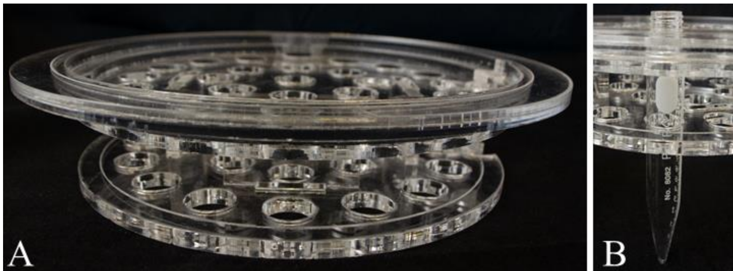
Figure S-1. Views of the assembled 15 mL glass tube support. (A) The assembled support alone. (B) The assembled support, elevated off the surface, with a tube in evaporation position, illustrating how the tube rests on the bottom of the bath.
