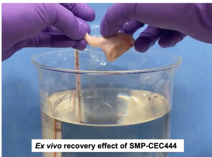
Figure S2. Shape-memory effect test videos. (a) In vitro simulation using a glass rod and (b) ex vivo simulation using the rat's hind limb.
