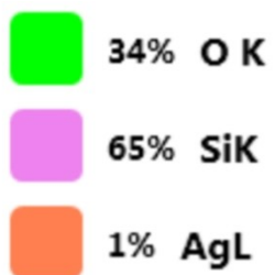
Figure S7: EDS - Elemental Mapping of SEM micrograph of SiIFoam. 65% Si and 34% O detected by EDS along with trace amounts of Ag (1%)
