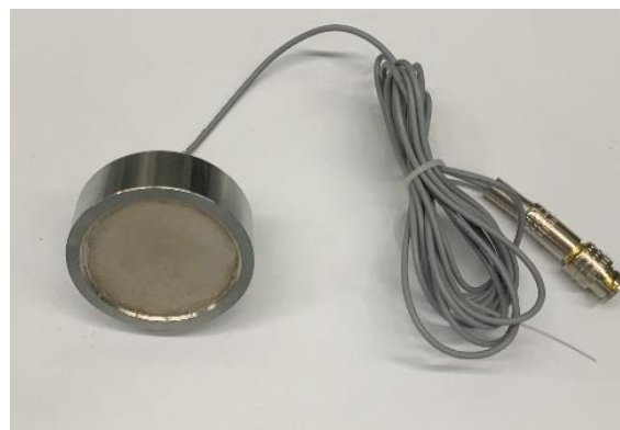
Fig S4. Focused ultrasonic probe is present.
