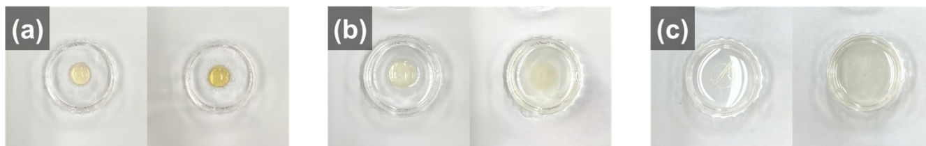
Fig. S3. Biodegradation of Casein_BLO (left) and Casein+TA_BLO (right) films in PBS solution (pH 7.4) at 37°C over time. Films were initially formed from 200 \mu L of precursor solution. (A) Day 0: immediately after immersion. (B) Day 1: partial degradation observed. (C) Day 2: complete degradation of both films, with only a faint outline remaining on the surface. PBS solution was replaced daily.
