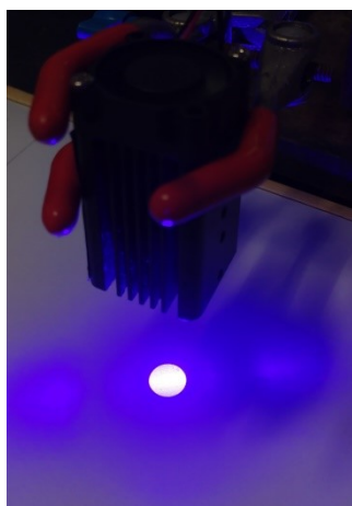
Figure S2. Digital photo of light instrument (Shanghai Zhuolong Electronics Co., Ltd, Shanghai, China), which can irradiate 450 nm light with same power density of 100 mW/cm 2 .
