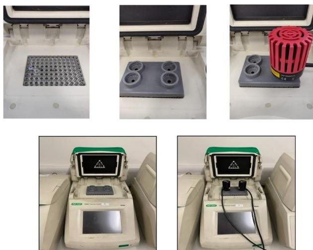
Figure S6. The UV cleavage apparatus used in this work. Using 3D-printing we have constructed a simple and inexpensive UV-irradiation device that sits on 96-well plates (or can be adapted to other formats). The device holds sample tubes at a fixed distance from the lamp to ensure consistent results. Between one and four LEDs of different wavelength can be used simultaneously (one and two lamps shown in the figure). In the present work just a single UV light source is required. Other designs can be readily constructed, and commercial systems are also available.
