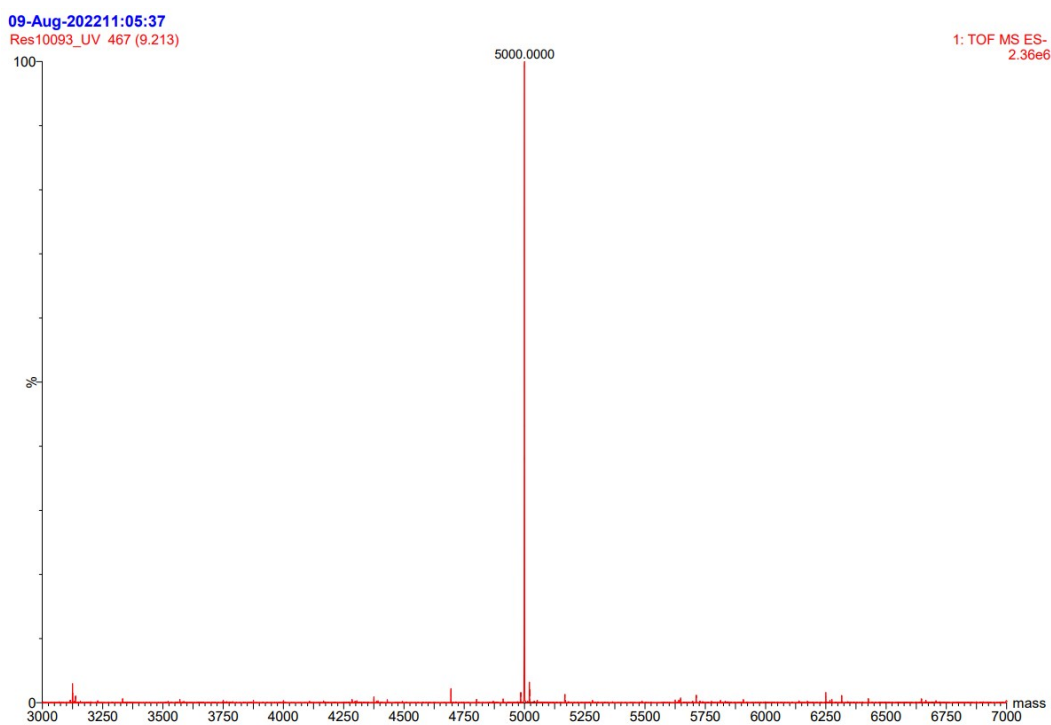
Figure S30. Mass spectrum of Cy3-ODN7UV. The calculated molecular weight is 4998.9 Da, and observed molecular weight is 5000 Da.
